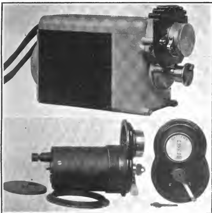
Samson unit starting, lighting and ignition system. Upper view shows complete unit and, lower, the dash coil and switch
